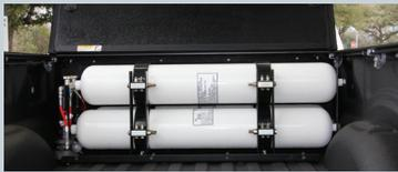
Activated carbon monoliths that allow low-pressure onboard natural gas fuel storage paired with conventional gasoline (bi-fuel hybrid).
