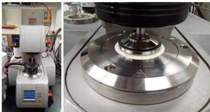
**Figure 3:** Modular compact rheometer (left) and full instrument profile (right) sample stage with a 50 mm parallel plate geometry.
