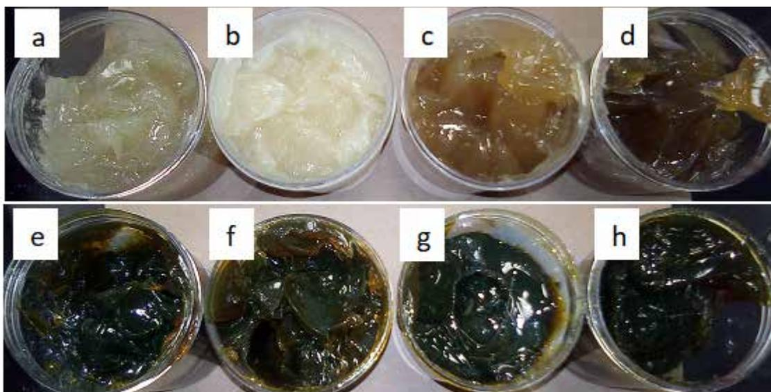
**Figure 5:** Grease samples using (top) NBO1 with (a) 12-HSA, (b) 12-HSA with azelaic acid, (c) MFA1, and (d) MFA2, and (bottom) NBO2 with (e) 12-HSA, (f) 12-HSA with azelaic acid, (g) MFA1, and (h) MFA2.
